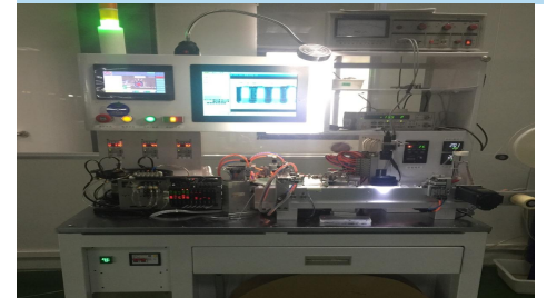
自动印字测试编带一体机 Automatic printing and testing taping all-in-one machine
