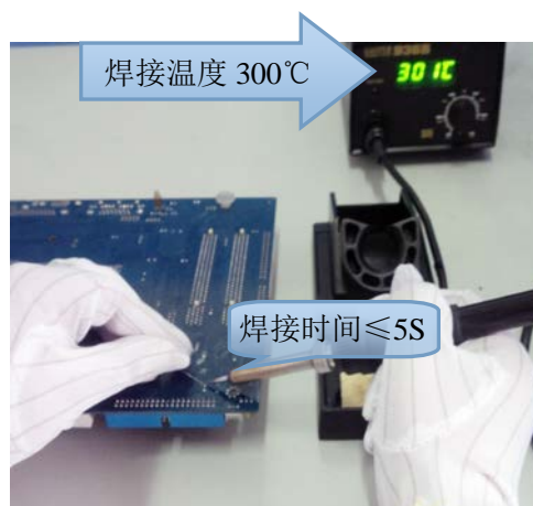
手工焊接 Manual Welding
